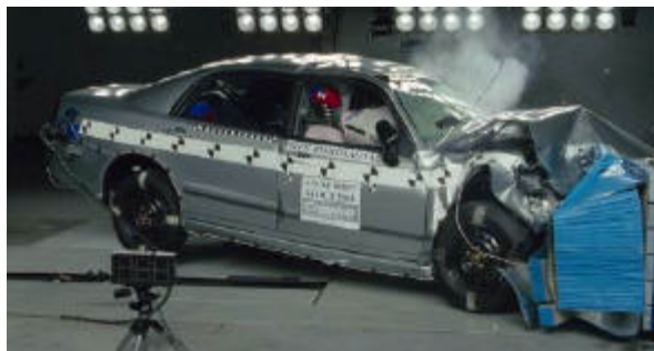
Offset crash test at 64km/h
