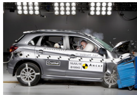
Frontal offset test at 64 km/h
