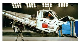
Offset crash test at 64km/h
