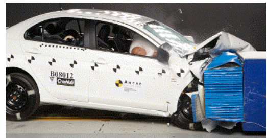
Offset crash test at 64km/h
