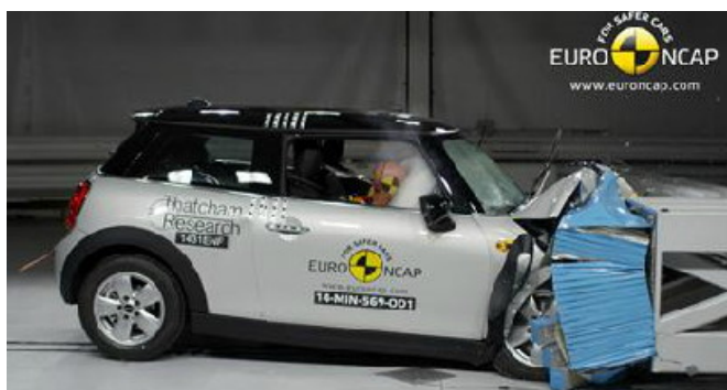
Frontal offset test at 64km/h
