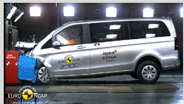
Frontal offset test at 56km/h (Mercedes-Benz V-Class)
