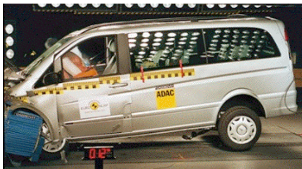
Offset crash test at 64km/h
