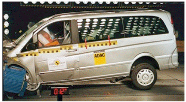
Offset crash test at 64km/h
