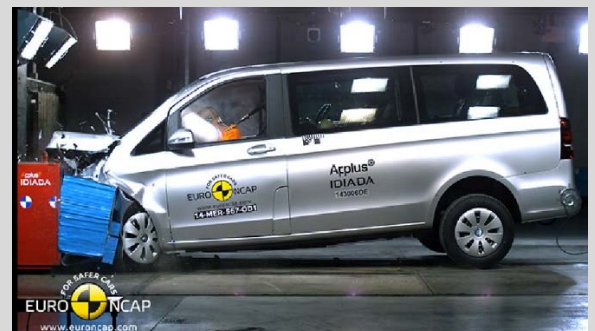
Frontal offset test at 56km/h
