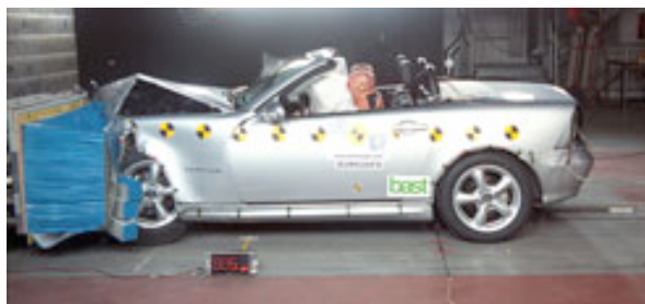
Offset crash test at 64km/h
