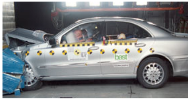
Offset crash test at 64km/h
