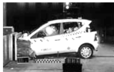
Offset crash test at 64km/h
