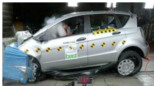
Offset crash test at 64km/h
