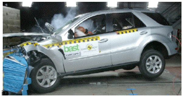
Offset crash test at 64km/h
