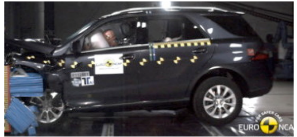
Offset crash test at 64km/h
