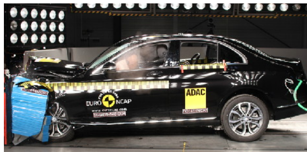
Frontal offset test at 64 km/h (Euro NCAP)
