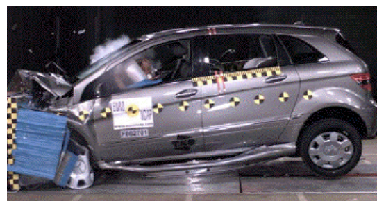
Offset crash test at 64km/h
