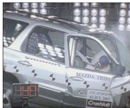
Offset crash test at 64km/h
