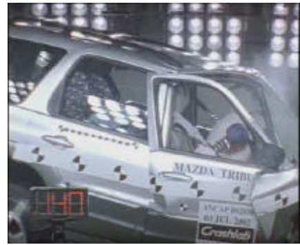
Offset crash test at 64km/h
