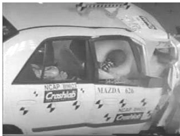
Offset crash test at 64km/h
