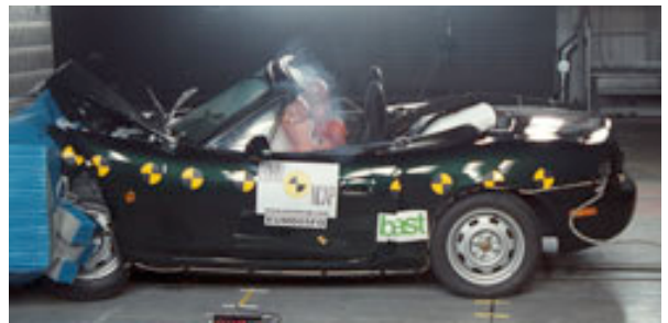
Offset crash test at 64km/h
