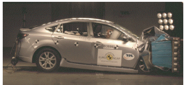
Offset crash test at 64km/h
