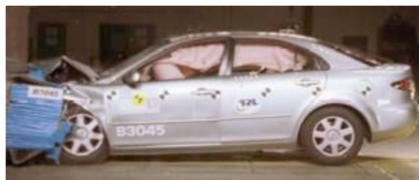
Offset crash test at 64km/h
