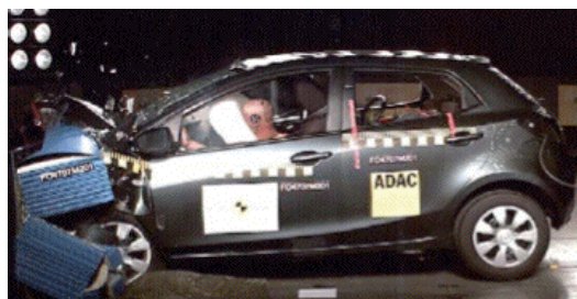
Offset crash test at 64km/h
