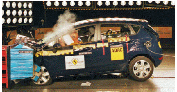
Offset crash test at 64km/h
