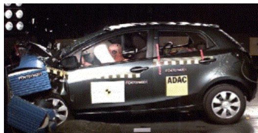
Offset crash test at 64km/h
