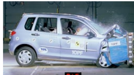
Offset crash test at 64km/h
