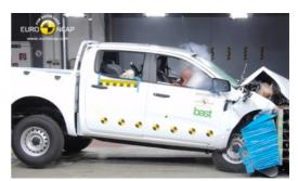
Offset crash test at 64km/h (Ford Ranger)
