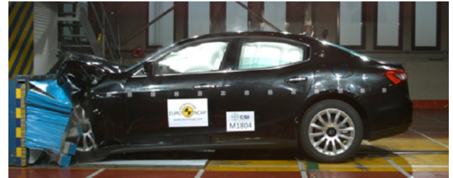
Frontal offset test at 64 km/h (Euro NCAP)
