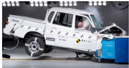
Offset crash test at 64km/h
