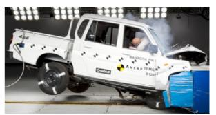
Offset crash test at 64km/h
