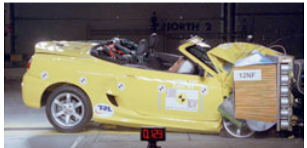
Offset crash test at 64km/h
