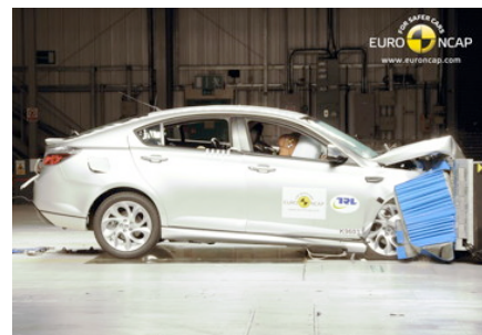
Frontal offset test at 64 km/h
