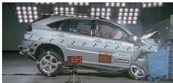
Offset crash test at 64km/h
