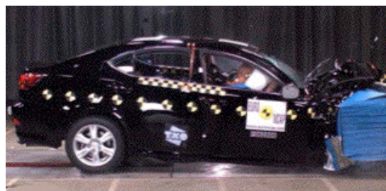
Offset crash test at 64km/h
