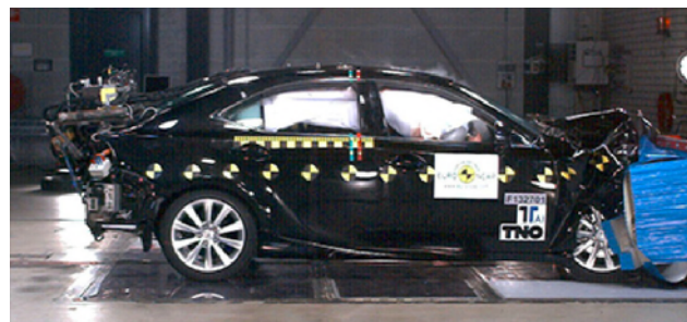
Frontal offset test at 64 km/h (Euro NCAP)
