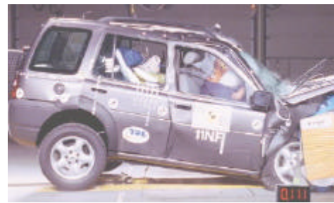
Offset crash test at 64km/h
