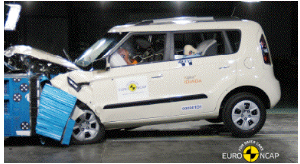
Offset crash test at 64km/h
