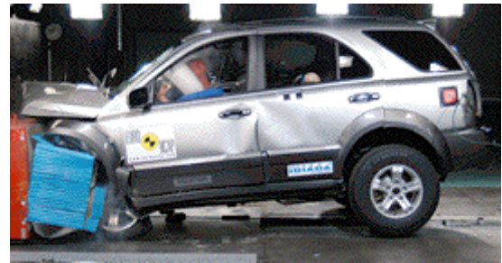
Offset crash test at 64km/h
