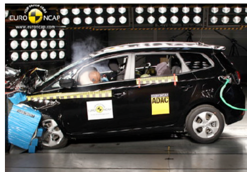
Frontal offset test at 64 km/h (Euro NCAP)
