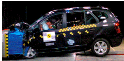
Offset crash test at 64km/h
