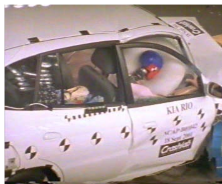
Offset crash test at 64km/h
