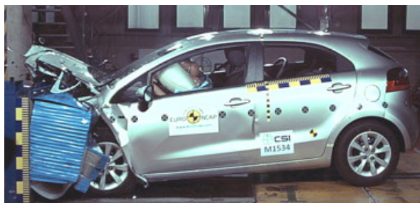
Offset crash test at 64km/h (Euro NCAP)
