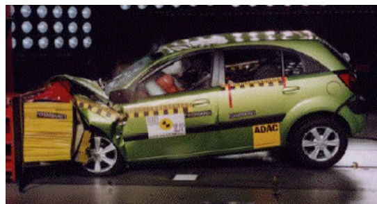
Offset crash test at 64km/h
