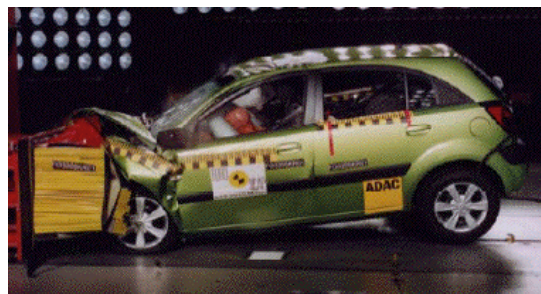
Offset crash test at 64km/h
