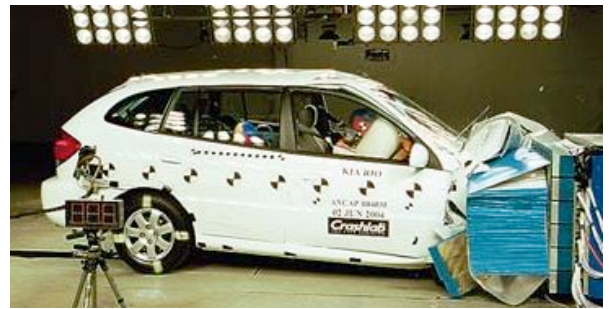
Offset crash test at 64km/h
