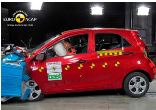
Frontal offset test at 64km/h
