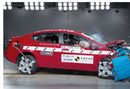
Frontal offset test at 64 km/h
