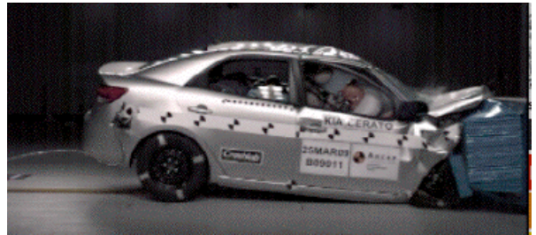
Offset crash test at 64km/h
