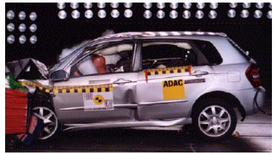
Offset crash test at 64km/h
